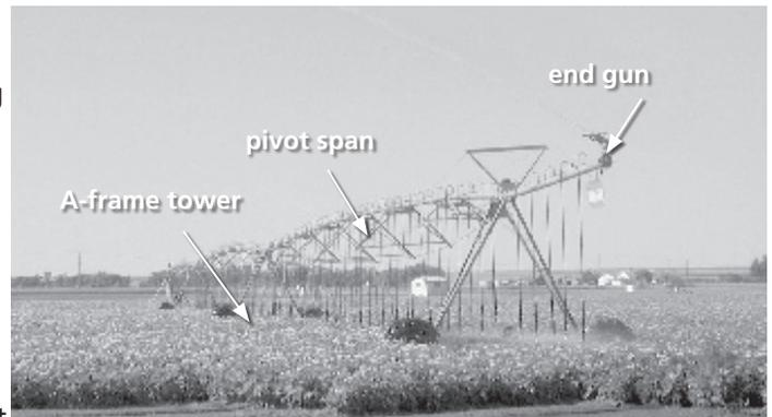
The system may vary in length from approximately 60 m to 790 m (200 to 2,600 ft.) and is capable of irrigating a circular area up to 200 ha (500 ac.). The most common system irrigates a circle of approximately 54 ha (133 ac.) of a square quarter section. Pressure required at the pivot may vary from approximately 70 kPa (10 psi) when low-pressure spray nozzles are used, to 550 kPa (80 psi) when high-pressure impact sprinklers are used.
