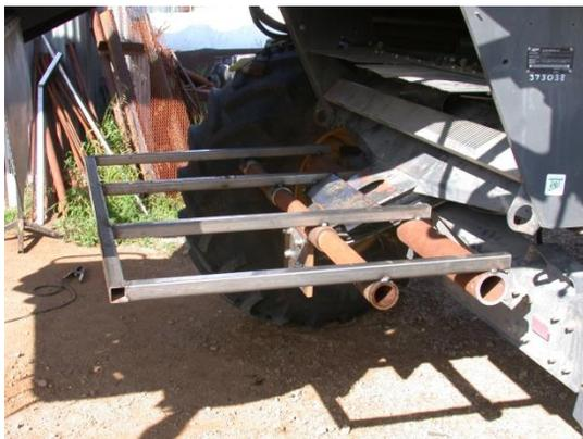
The frame behind the hinge point is heavier than necessary. This requires more counter balance weight on the front to reset the box.
