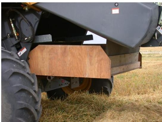
Finished chaff box. Note the back door hanging from the combine frame, and the chaff pan extension made with galvanized tin.
