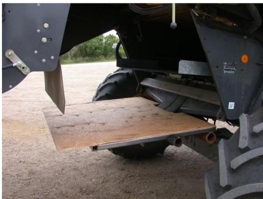
Quarter inch plywood floor bolted to the frame.
